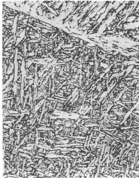
Figure 9 Microstructure of the weld metal with larger prior austenite grain size at 4^{\circ}\text{C s}^{-1} ( 208\ \mu\text{m} ), \times 500
