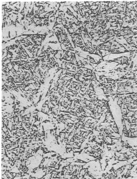
Figure 8 Microstructure of the weld metal with medium prior austenite grain size at 4^{\circ}\text{C s}^{-1} ( 93\ \mu\text{m} ), \times 500
